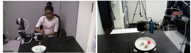
Figure 1: Eye gaze detected in real time through a worn eye tracker can reveal human mental states and guide robot assistance in human-robot shared manipulation tasks.
